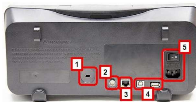
Picture 1.1-3 Back panel connection locations on SDS1000CF series
