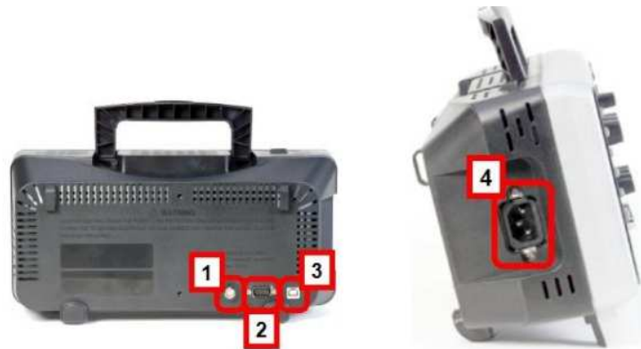
Picture 1.1-4 Back and Side panel connection locations on SDS1000C/CM/CE Series oscilloscope.
